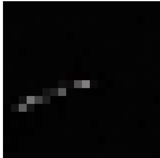
Figure 3. Examples of images taken with the completely covered camera of a smartphone using the CREDO application.
